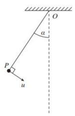
The diagram shows a particle P, of mass m, which is attached by a light inextensible string, of length l, to a fixed support O. The particle moves in a vertical plane. It is initially set in motion with speed u at right angles to OP, from the position where OP makes an angle  $\alpha$  with the downward vertical through O.
