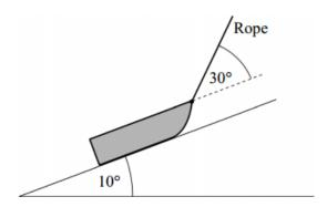
Find the acceleration of the sledge if the tension in the rope is 60 N.
