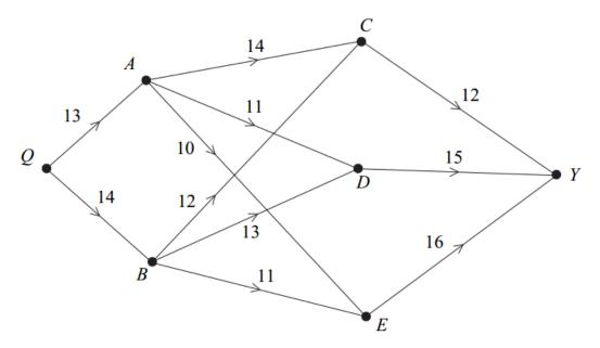
The truck is able to carry a load of up to 20 tonnes. The optimal route, known as the maximin route, is that for which the possible load that the truck can carry is as large as possible.
